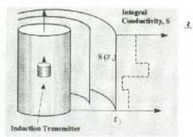
A few cylindrical surfaces of heterogeneous integral conductivity are placed in surrounding formation. Excitation device is point or finite induction transmitter producing axial magnetic field. The primary current changes due to harmonic or transient regime. Model is oriented to study problems dealing with casing and metrology of logging instruments.
