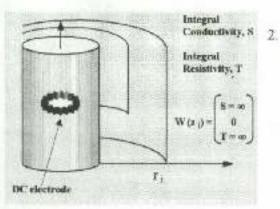
Medium contains a set of cylindrical envelopes with piecewise uniform distribution of shielding electrical property ("reflecting", "transparent" and "absorbing" thin sheet). The source of incident direct current is point or circular electrode. This synthetic model is a basic for development of physical substantiation and numerical algorithm.
